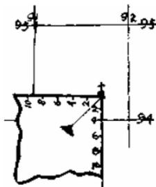
To use, place the square corner on the point you wish to give or find map reference for with edges parallel to side of grid squares. Read scale where cut by grid lines, (figure 3). This reading is 919944. Remember to read across (Easting) and up (Northing). Go in the door and then upstairs is an easy way to remind yourself.
