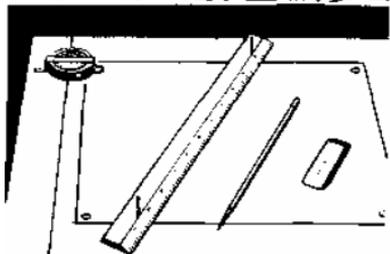
For sighting you need a sight ruler, an "alidade". Use an ordinary ruler with 2 finishing nails driven in at either end and same distance from edge of ruler.
