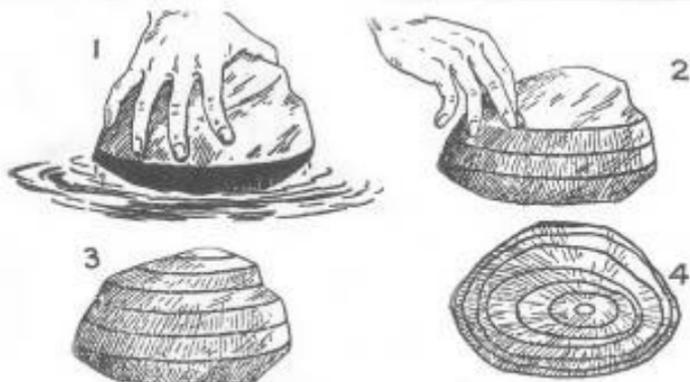
Another way to demonstrate contour lines simply is to dip a rock part way in water and draw the water line. Dip one inch deeper; draw another line and so on. The diagram above shows this method.
